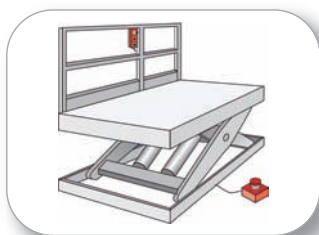
Push button control on the railing
