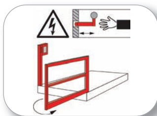
Full gate with mechanical lock and interlock
