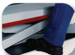
Additional foot protection contact strip on the scissor leg
