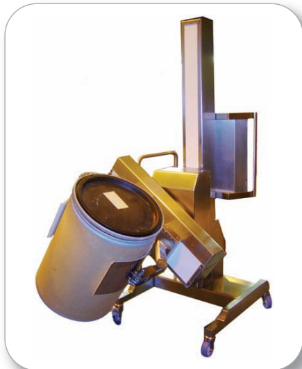
Manual push, powered lift, grip and pour
