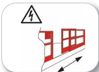
Sliding gate in the railing, width 800 mm, table length 2m min. (door side)
