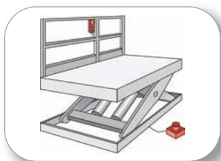
Push button control on the railing
