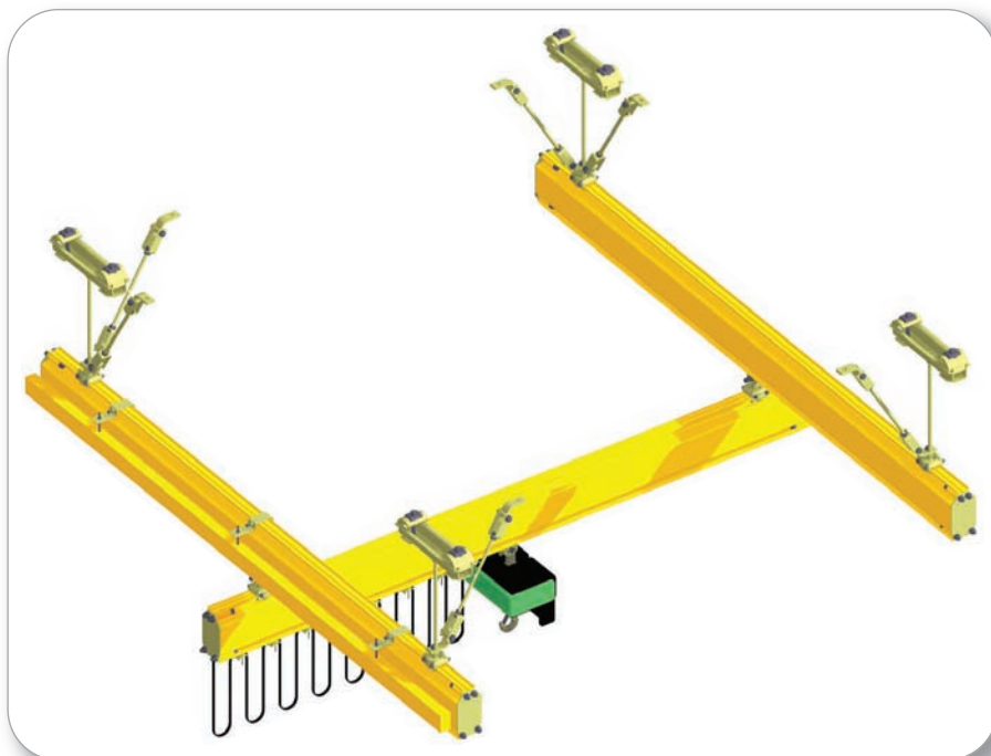
Single Girder Articulated Crane
